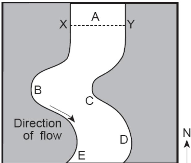
168 At which two locations in this stream is deposition normally dominant over erosion?
